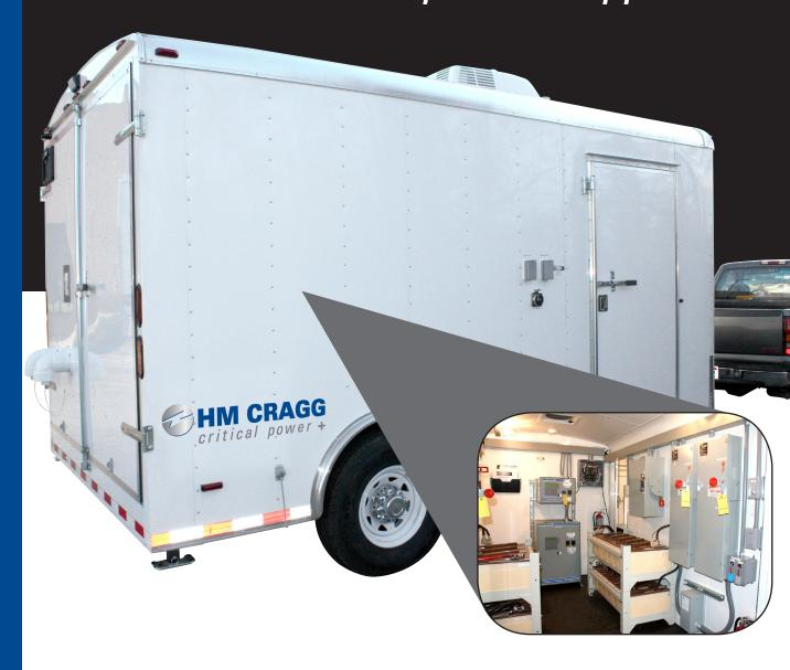
Designed, engineered and built by HM Cragg, the MOBILE POWER SYSTEM caters to electric utility, outdoor event and telecommunications applications. Each unit is customized to meet the specifications and system requirements of the customer.
